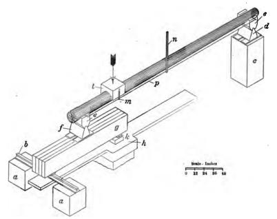
Fig. 45.—Method of testing poles.
